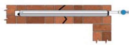
Stitching a cracked solid wall
