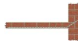
5 Reconnecting internal walls with external walls
