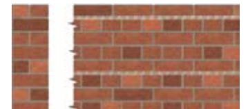
8 Creating masonry beams
