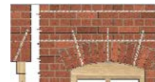
2 Repairing brick arch lintels
