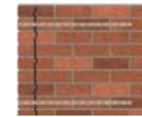
3 Repairing cracks near corners and openings
